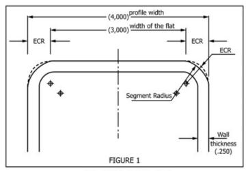
$$ECR = \frac{\text{(Tube Width)} - \text{(Width of Flat)}}{2}$$
